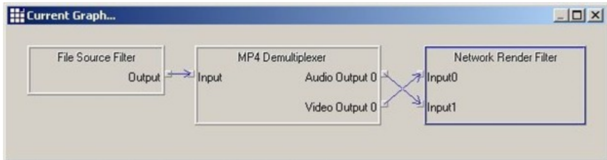
Figure 17. Filter Graph for MP4 File Broadcasting
