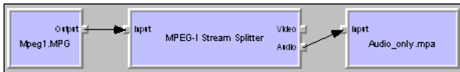
Figure 1. Audio Stream Splitting and Dumping to a File
